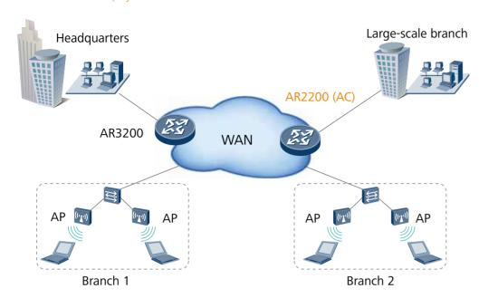
The AR2200 routers integrate AC (Access Controller) functionality, which can manage the wireless AP (Access Point) in wireless LAN. AR2200 supports rich certification and flexible user access control, which can provide security access guarantee for Wi-Fi users. The rich wireless capabilities integrated in one device, this can realize centralized management of wired and wireless networks, to meet the requirements of different scale enterprises networks.
