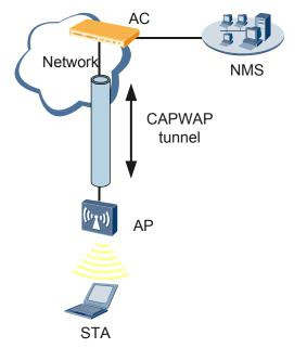
APs establish CAPWAP tunnels with the AC, including the data tunnel and control tunnel.
