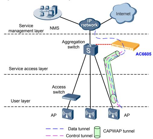
Figure 2-3 Centralized data forwarding
