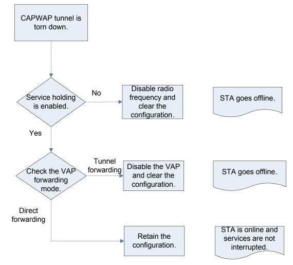
Figure 2-5 Implementation of service holding upon CAPWAP link disconnection
