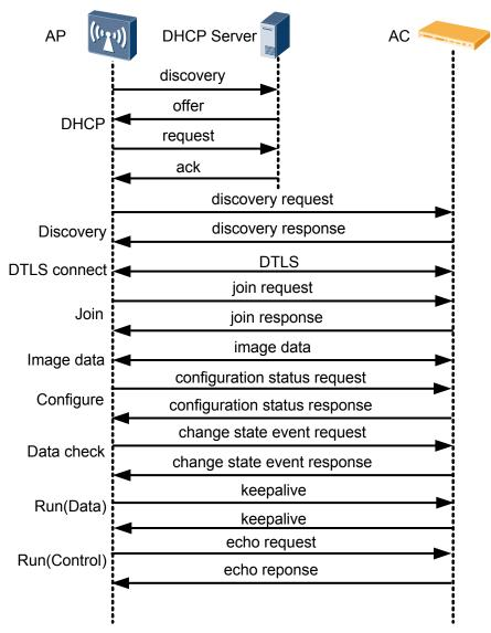
Figure 2-2 CAPWAP tunnel establishment
