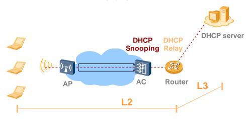
When a WLAN AC functions as a Layer 2 switch for STAs, you can enable the DHCPv6 SNP function to obtain the IPv6 addresses allocated to STAs and provide support for IPv6 SG.
