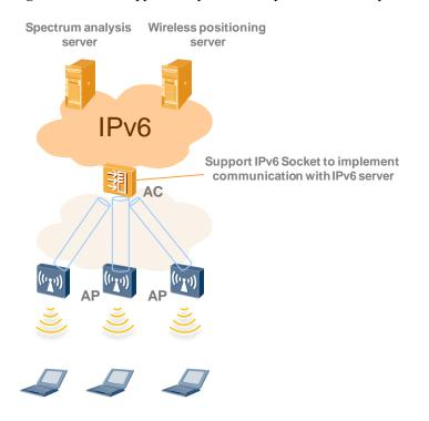
Figure 2-16 IPv6 support for spectrum analysis and wireless positioning
