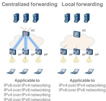
Figure 2-2 WLAN centralized forwarding and local forwarding
