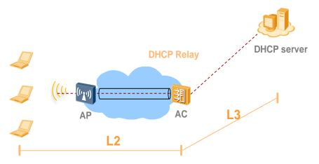
If a WLAN AC functions only as a Layer 2 switch for STAs, you can deploy the DHCPv6 relay function on the upstream router to allocate IPv6 addresses to STAs, as shown in Figure 2-15.
