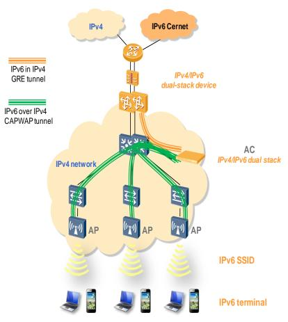
Figure 4-1 Dual-stack network solution
