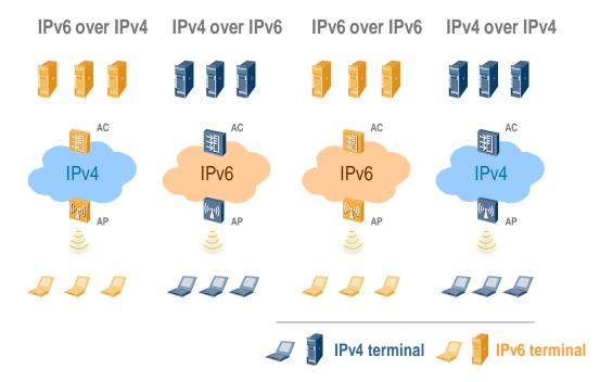
Figure 2-1 WLAN IPv4/IPv6 networking modes
