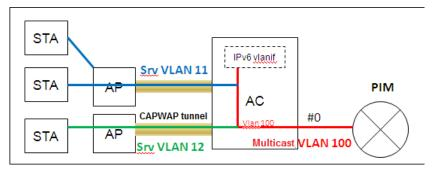
In IPv6 multicast VLAN, different VAPs use different service VLANs (Srv VLANs for short) but correspond to the same upstream multicast VLAN. This feature is the same as IPv4 multicast VLAN. Allocation requirements of this feature are as follows: WLAN DBSS virtual interfaces must support multicast VLAN.
