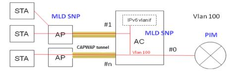
Figure 2-8 WLAN IPv6 multicast
