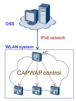
IPv4/IPv6 dual-stack WLAN products can be directly managed by the OSS, which is the IPv6 network management platform. In the Infrastructure WLAN, an AC provides the network management interface; the OSS performs network management control on the AC; the AC manages and controls all the APs through CAPWAP control channels. That is, only the AC has network management channels, but APs do not have independent network management channels.
