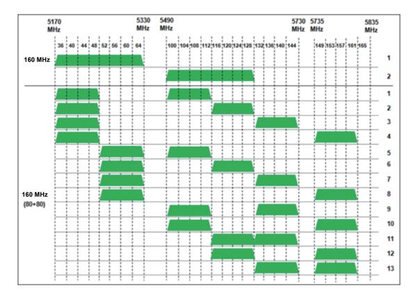
Wider channel bonding can provide wider channel bandwidth. Channel bonding helps avoid some interference and can improve the utilization of scattered channels.
