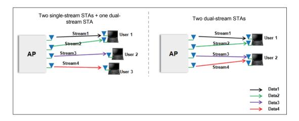
MU-MIMO is an outstanding feature of 802.11ac Wave 2, which depends on explicit transmit beamforming (TxBF). This feature requires that STAs support explicit TxBF. The reason is that when an AP concurrently transmits data to multiple users over the same frequency, signals are interference to users who are not target receivers of the signals. MU-MIMO uses TxBF to detect channels and uses precoding technology based on the feedback to mitigate such interference.
