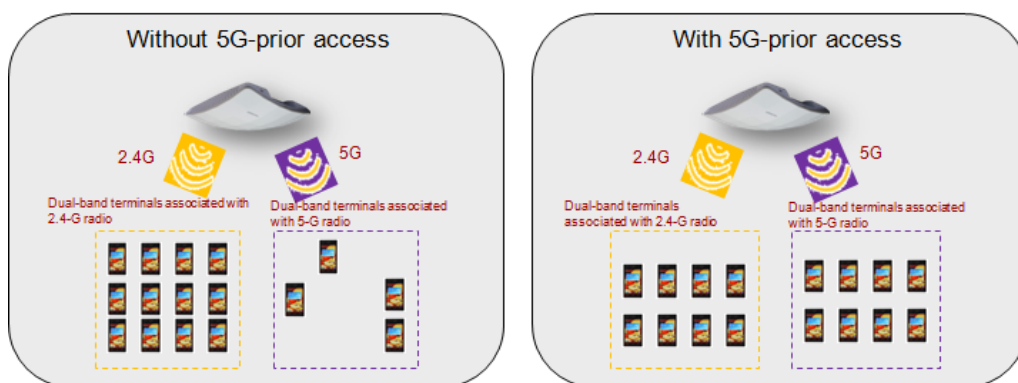
Figure 2-12 Load balancing between radios
