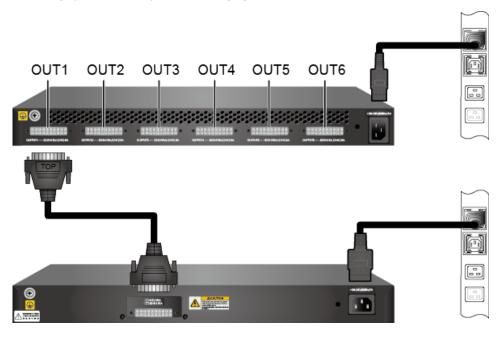
The RPS1800 can connect to a maximum of six switches and ensures seamless failover for at most one switch when the internal power supply of the switch fails.
