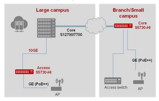
Huawei S5730-HI is the next-generation fixed agile switch. The S5730-HI has large table sizes and buffers, avoiding packet loss in traffic bursts. It supports wired and wireless convergence and unified management on devices, users, and services. The S5730-HI can be used as the core device on an enterprise branch network or a small campus network or as the aggregation or
