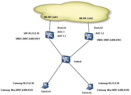
Figure 3-1 Typical GLBP networking diagram
