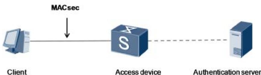
Figure 2-1 Point-to-point connection between a host and network device
