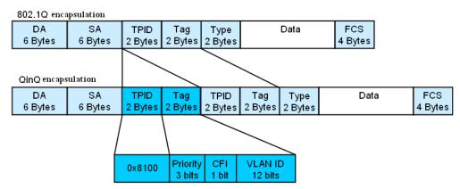
Figure 7-1 Format of QinQ packets
