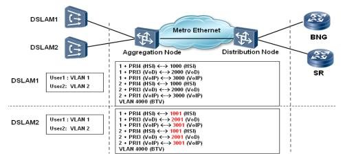
Figure 8-2 VLAN mapping based on VLAN IDs and priorities
