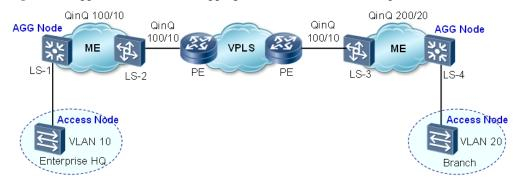
Figure 8-4 Application of VLAN mapping and selective QinQ in enterprise leased lines
