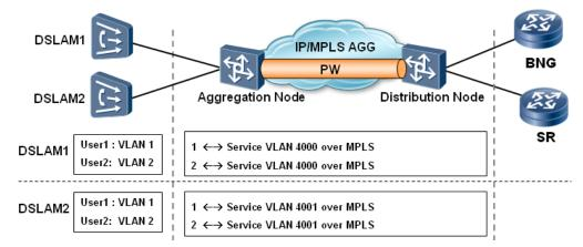
Figure 8-3 Application of VLL/VPLS after VLAN mapping
