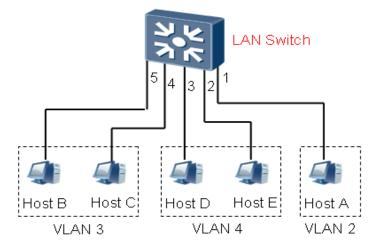
Figure 6-1 MUX VLAN networking
