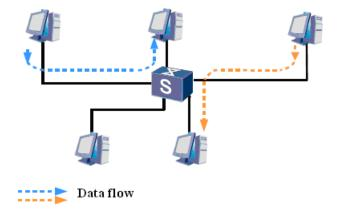
Figure 1-2 L2 switch networking
