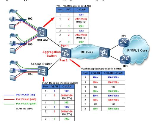
Figure 8-1 Application of VLAN Mapping and Selective QinQ in MANs
