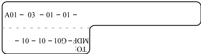
Figure 5-92 Example of labels for user cables
