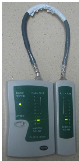
Figure 5-39 Testing the conduction and connections of wires
