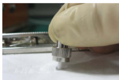
Figure 5-96 Cleaning optical fibers with special cleaning tissues
