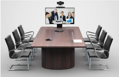
The HUAWEI TE30 videoconferencing endpoint (TE30 for short) delivers 1080p HD video performance in a sleek design.
